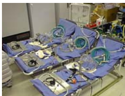
Suit simulator set up for multiple semi-recumbent intermittent light exercise simulating astronaut tasks
